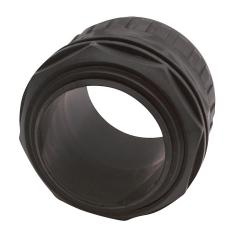
Iboco connector, liquid-tight, straight, 2in trade size, G2 BSPP thread type, black. Package of 5. For use with I-Flex electrical tubing. Seal gaskets included.
