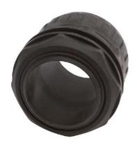
Iboco connector, liquid-tight, straight, 1-1/2in trade size, G1-1/2 BSPP thread type, black. Package of 5. For use with I-Flex electrical tubing. Seal gaskets included.
