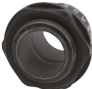
Iboco connector, liquid-tight, straight, 1-1/4in trade size, G1-1/4 BSPP thread type, black. Package of 10. For use with I-Flex electrical tubing. Seal gaskets included.
