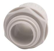
Iboco connector, liquid-tight, straight, 1in trade size, G1 BSPP thread type, gray. Package of 10. For use with I-Flex electrical tubing. Seal gaskets included.
