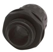
Iboco connector, liquid-tight, straight, 3/4in trade size, G3/4 BSPP thread type, black. Package of 20. For use with I-Flex electrical tubing. Seal gaskets included.
