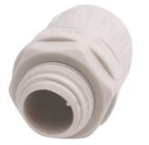
Iboco connector, liquid-tight, straight, 1/2in trade size, G1/2 BSPP thread type, gray. Package of 20. For use with I-Flex electrical tubing. Seal gaskets included.
