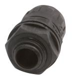
Iboco connector, liquid-tight, straight, 3/8in trade size, G3/8 BSPP thread type, black. Package of 20. For use with I-Flex electrical tubing. Seal gaskets included.
