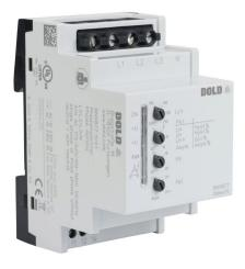
Dold phase monitor relay, 3-phase, 35mm DIN rail mount, 175-525 VAC input voltage, SPDT, 5A contact rating, screw terminal(s), LED indicator(s), phase reversal, phase unbalance, overvoltage, undervoltage, voltage range and neutral protection.
