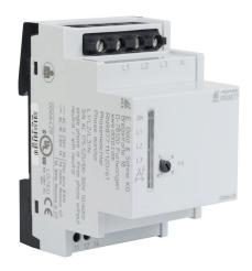
Dold phase monitor relay, 3-phase, 35mm DIN rail mount, 175-525 VAC input voltage, SPDT, 5A contact rating, screw terminal(s), LED indicator(s), phase reversal, phase loss and phase unbalance protection.
