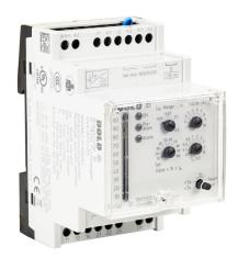
Dold residual current monitor, 10 mA to 3A selectable trip point, voltage and relay, (2) SPDT, normally energized or normally deenergized, manual reset output, 80-230 VAC/VDC operating voltage. Requires Dold ND5015-070-61 transformer.
