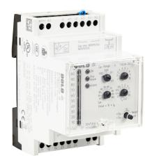
Dold residual current monitor, 10 mA to 3A selectable trip point, voltage and relay, (2) SPDT, normally energized or normally deenergized, manual reset output, 80-230 VAC/VDC operating voltage. Requires Dold ND5015-24-61 or ND5015-35-61 transformers.
