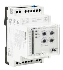
Dold residual current monitor, 10 mA to 3A selectable trip point, voltage and relay, (2) SPDT, normally energized or normally deenergized, manual reset output, 24-80 VAC/VDC operating voltage. Requires Dold ND5015-24-61 or ND5015-35-61 transformers.
