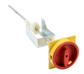
WEG Electric rotary handle, selector, red/yellow, external front mount, 2-position, lockable in OFF only, NEMA 1/3R, IP55. For use with MPW40 series manual motor protectors. 330mm shaft included.
