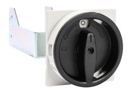
WEG Electric rotary handle, selector, black/gray, external front mount, 2-position, lockable in OFF only, NEMA 1/3R, IP55. For use with MPW40 series manual motor protectors. 130mm shaft included.
