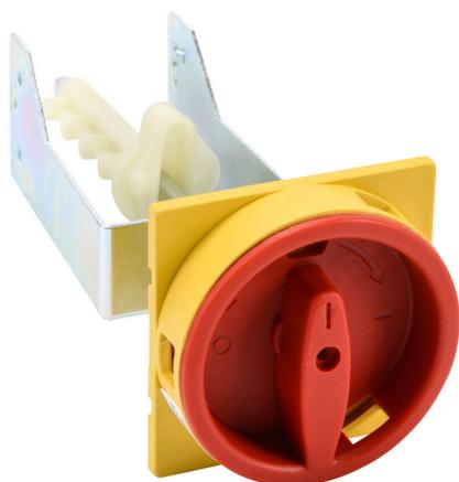
WEG Electric rotary handle, selector, red/yellow, external front mount, 2-position, lockable in OFF only, NEMA 1/3R, IP55. For use with MPW40 series manual motor protectors. 130mm shaft included.
