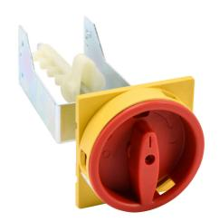
WEG Electric rotary handle, selector, red/yellow, external front mount, 2-position, lockable in OFF only, NEMA 1/3R, IP55. For use with MPW40 series manual motor protectors. 130mm shaft included.
