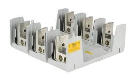
Bussmann modular fuse block, accepts R fuses, 600A, 600V, 3-pole, 2 line/2 load opening(s) per pole, (2) 4 AWG-500 MCM copper or aluminum, box lug, panel mount.
