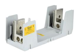
Bussmann modular fuse block, accepts R fuses, 600A, 600V, 1-pole, 2 line/2 load opening(s) per pole, (2) 4 AWG-500 MCM copper or aluminum, box lug, panel mount.
