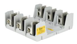
Bussmann modular fuse block, accepts R fuses, 400A, 600V, 3-pole, 4 AWG-600 MCM copper or aluminum, box lug, panel mount.
