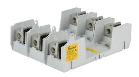
Bussmann modular fuse block, accepts R fuses, 200A, 600V, 3-pole, 6 AWG-250 MCM copper or aluminum, box lug, panel mount.
