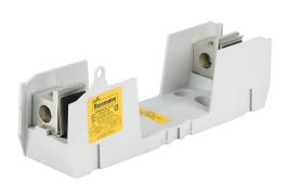
Bussmann modular fuse block, accepts R fuses, 200A, 600V, 1-pole, 6 AWG-250 MCM copper or aluminum, box lug, panel mount
