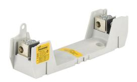
Bussmann modular fuse block, accepts R fuses, 100A, 600V, 1-pole, 14-1/0 AWG copper or aluminum, box lug, panel mount.
