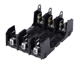
Bussmann modular fuse block, accepts R fuses, 60A, 600V, 3-pole, 14-2 AWG copper or 8-2 AWG aluminum, box lug, 35mm DIN rail or panel mount.
