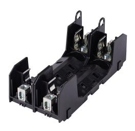
Bussmann modular fuse block, accepts R fuses, 60A, 600V, 2-pole, 14-2 AWG copper or 8-2 AWG aluminum, box lug, 35mm DIN rail or panel mount.
