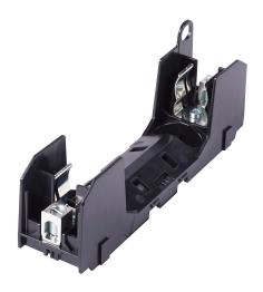
Bussmann modular fuse block, accepts R fuses, 60A, 600V, 1-pole, 14-2 AWG copper or 8-2 AWG aluminum, box lug, 35mm DIN rail or panel mount.
