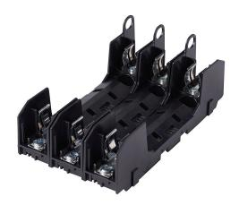
Bussmann modular fuse block, accepts R fuses, 30A, 600V, 3-pole, 18-10 AWG copper only, screw with pressure plate, 35mm DIN rail or panel mount.
