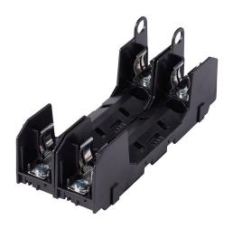
Bussmann modular fuse block, accepts R fuses, 30A, 600V, 2-pole, 18-10 AWG copper only, screw with pressure plate, 35mm DIN rail or panel mount.
