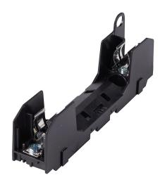
Bussmann modular fuse block, accepts R fuses, 30A, 600V, 1-pole, 18-10 AWG copper only, screw with pressure plate, 35mm DIN rail or panel mount.
