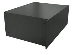
Hammond enclosure, 4U, 7 x 17 x 13in (HxWxD), rack or desktop mount, aluminum, black, powder coat finish, screw cover.
