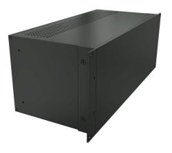
Hammond enclosure, 4U, vented, 7 x 17 x 8in (HxWxD), rack or desktop mount, aluminum, black, powder coat finish, screw cover.
