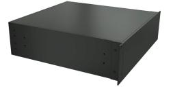
Hammond enclosure, 3U, 5 x 17 x 18in (HxWxD), rack or desktop mount, aluminum, black, powder coat finish, screw cover.
