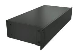
Hammond enclosure, 2U, 4 x 17 x 8in (HxWxD), rack or desktop mount, aluminum, black, powder coat finish, screw cover.
