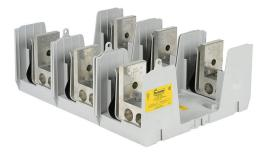
Bussmann modular fuse block, accepts R fuses, 600A, 250V, 3-pole, 2 line/2 load opening(s) per pole, (2) 4 AWG-500 MCM copper or aluminum, box lug, panel mount.
