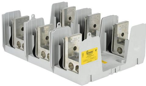
Bussmann modular fuse block, accepts R fuses, 600A, 250V, 3-pole, 2 line/2 load opening(s) per pole, (2) 4 AWG-500 MCM copper or aluminum, box lug, panel mount.
