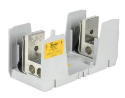
Bussmann modular fuse block, accepts R fuses, 600A, 250V, 1-pole, 2 line/2 load opening(s) per pole, (2) 4 AWG-500 MCM copper or aluminum, box lug, panel mount.
