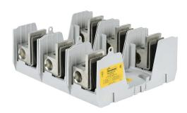
Bussmann modular fuse block, accepts R fuses, 400A, 250V, 3-pole, 4 AWG-600 MCM copper or aluminum, box lug, panel mount.
