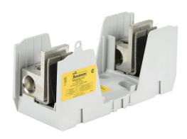
Bussmann modular fuse block, accepts R fuses, 400A, 250V, 1-pole, 4 AWG-600 MCM copper or aluminum, box lug, panel mount.
