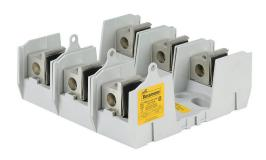
Bussmann modular fuse block, accepts R fuses, 200A, 250V, 3-pole, 6 AWG-250 MCM copper or aluminum, box lug, panel mount.
