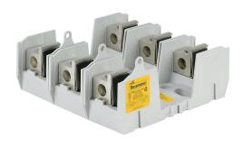
Bussmann modular fuse block, accepts R fuses, 200A, 250V, 3-pole, 6 AWG-250 MCM copper or aluminum, box lug, panel mount.
