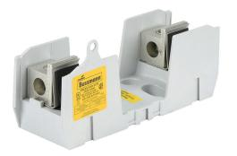
Bussmann modular fuse block, accepts R fuses, 200A, 250V, 1-pole, 6 AWG-250 MCM copper or aluminum, box lug, panel mount.
