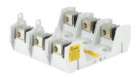
Bussmann modular fuse block, accepts R fuses, 100A, 250V, 3-pole, 14-1/0 AWG copper or aluminum, box lug, panel mount.
