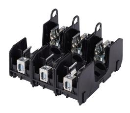
Bussmann modular fuse block, accepts R fuses, 60A, 250V, 3-pole, 14-2 AWG copper or 8-2 AWG aluminum, box lug, 35mm DIN rail or panel mount.
