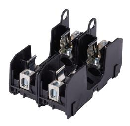
Bussmann modular fuse block, accepts R fuses, 60A, 250V, 2-pole, 14-2 AWG copper or 8-2 AWG aluminum, box lug, 35mm DIN rail or panel mount.
