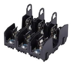
Bussmann modular fuse block, accepts R fuses, 30A, 250V, 3-pole, 18-10 AWG copper only, screw with pressure plate, 35mm DIN rail or panel mount.
