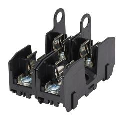
Bussmann modular fuse block, accepts R fuses, 30A, 250V, 2-pole, 18-10 AWG copper only, screw with pressure plate, 35mm DIN rail or panel mount.
