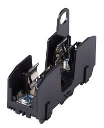
Bussmann modular fuse block, accepts R fuses, 30A, 250V, 1-pole, 18-10 AWG copper only, screw with pressure plate, 35mm DIN rail or panel mount.
