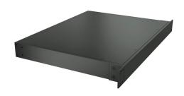
Hammond enclosure, 1U, 2 x 17 x 13in (HxWxD), rack or desktop mount, aluminum, black, powder coat finish, screw cover.
