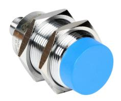
Contrinex RFID read-write module, tubular, non-flush mount, HF communication, 13.56 MHz, 58mm read-write distance, (1) 4-pin M12 A-coded (IO-Link) port(s), IO-Link Class A Device, 30mm diameter x 63.5mm body, IP67.
