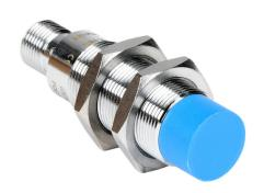
Contrinex RFID read-write module, tubular, non-flush mount, HF communication, 13.56 MHz, 26mm read-write distance, (1) 4-pin M12 A-coded (IO-Link) port(s), IO-Link Class A Device, 18mm diameter x 63.5mm body, IP67.
