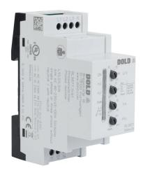
Dold phase monitor relay, 3-phase, 35mm DIN rail mount, 80-230 VAC input voltage, SPDT, 5A contact rating, screw terminal(s), LED indicator(s), phase reversal, phase unbalance, overvoltage, undervoltage, voltage range and neutral protection.
