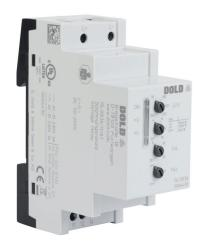
Dold voltage monitor relay, 1-phase, 35mm DIN rail mount, 50-250 VDC input voltage, SPDT, 5A contact rating, screw terminal(s), LED indicator(s), overvoltage, undervoltage and voltage range protection.
