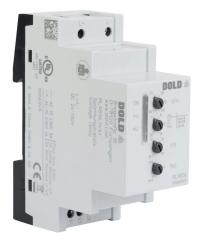
Dold voltage monitor relay, 1-phase, 35mm DIN rail mount, 24-130 VDC input voltage, SPDT, 5A contact rating, screw terminal(s), LED indicator(s), overvoltage, undervoltage and voltage range protection.
