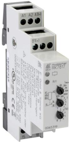
Dold multi-mode relay timer, 0.02 seconds to 300 hours selectable timing range, 24 VAC/VDC and 110-127 VAC operating voltage, 2A contact rating, (1) SPDT timed relay output(s), 35mm DIN rail mount, screw terminal(s).
